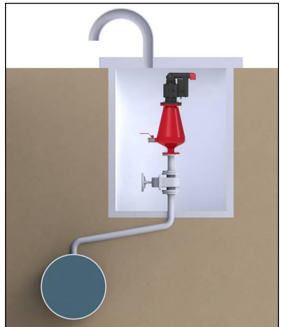
Two Air Valves on a shared Isolating Valve. Air Valves outlets face outward and the Isolating Valve at 45° to Air Valve outlets
