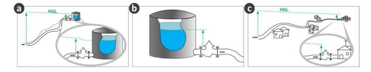
\* HGL: Hydraulic Grade Line - the line representing the available head (sum of the pressure and elevation) at any point in the system.
