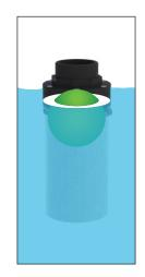
When the float reaches the sealing seat, it closes the Flood Guard drip-tight, preventing the intake of contaminated water.
