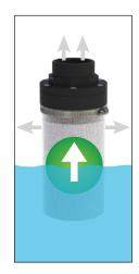
If the flood level continues to rise, the float of the Flood Guard will rise with the buoyant force.
