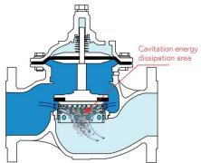
Anti-Cavitation Air-Suction: This is a unique solution provided as an optional feature in DOROT S100 control valves. Special air-suction devices allow jets of atmospheric air to enter the low-pressure area in the vena-contracta, thus preventing the pressure from dropping below the vapor pressure,
