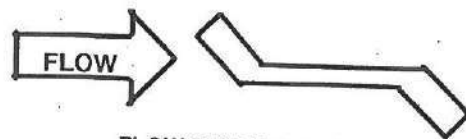
FLOW UNDER SEAT DIAPHRAGM FAILURE = VALVE FAILS TO CLOSE
