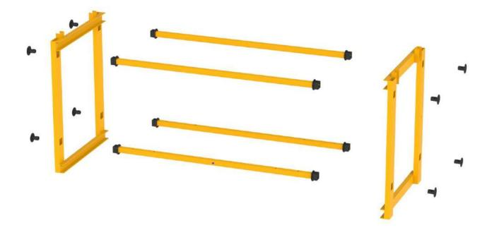
3. Note the skid positioning direction (note the location of the connecting rods sockets) and place the first frame it that direction. Note that the right frame is marked with a green sticker, and the left frame is marked with a red sticker.
