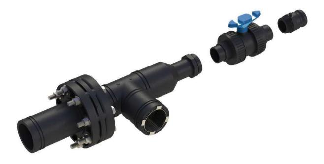
3. Assemble the outlet manifold: Assemble a 2" ball valve to the Outlet Pipe, and a 2" camlock adaptor to the ball valve.
