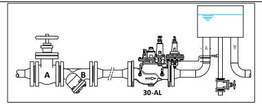
a. The valve can be installed in any position, although installation with the bonnet facing up is recommended for ease of maintenance. b. Flow direction should match the engraved arrow on the bonnet.
