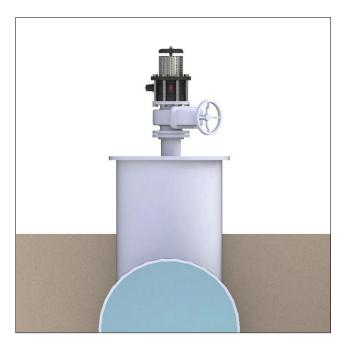
Single Vacuum Breaker on an Isolating Valve at 45° to Air Valve
