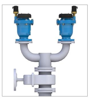
Two Air Valves on a shared Isolating Valve. Air Valves outlets face outward and the Isolating Valve at 45° to Air Valve outlets
